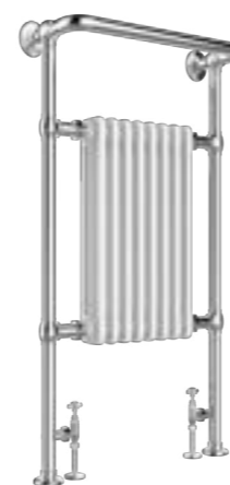
Grosvenor Size: 963 x 673 x 230 Bars: 8 BTU: 3410 Pipe Center: 438mm Projection: 230mm Recommended Element: 600W Chrome GRO963CW £520.00
